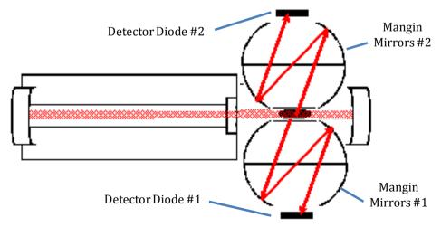
Fig 2. HeNe Active Cavity Optical Bench- Side View, (air flow is towards the reader)
