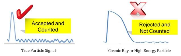
Fig 11. Dark Particle Rejection using Field Programmable Gate Array FPGA
