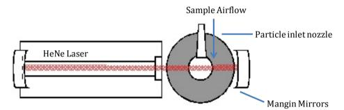
Fig 1. HeNe Active Cavity Optical Bench- Top View
