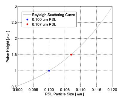
Fig 4. Rayleigh Scattering Curve or 0.100 and 0.107 μm Particles
