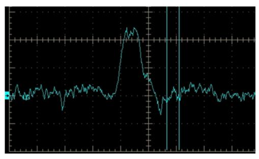
Fig 5. A typical 0.100 μm Particle Signal Pulse Taken from a Single Detector Element
