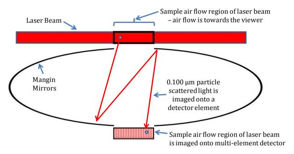
Fig 9. Laser Beam is sharply focused onto the Multi Element Detector
