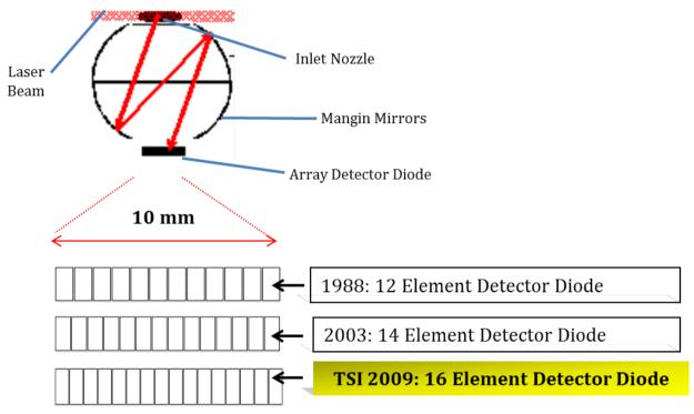
Fig 8. Detector Diode Evolution
